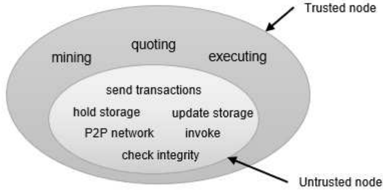
Figure 5: Relations between trusted node and untrusted node
